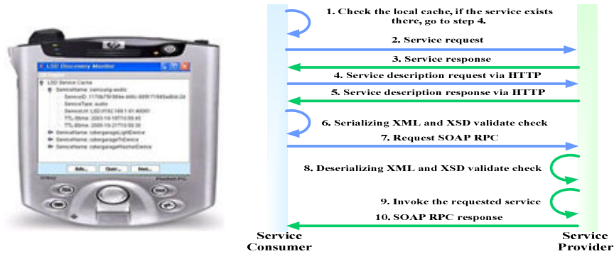
Fig. 7. A Sequence Diagram of remote data access scheme in LSD
